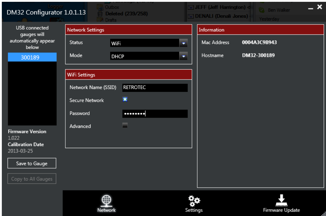
Figure 19: Secure WiFi network needs DHCP, Network name, and Password entered
